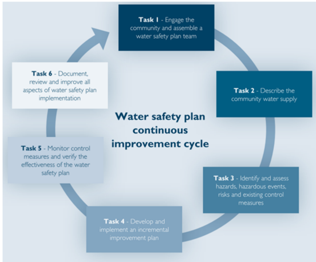
Figure 8: The six tasks to develop and implement a water safety plan in a small community water supply.
